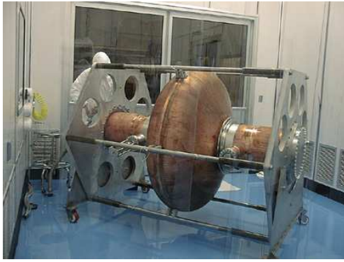
Figure 2: 200MHz cavity on a horizontal supporting frame.
