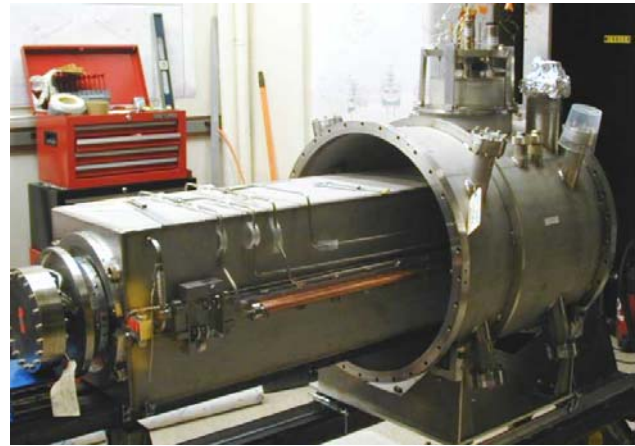
Figure 3: Cold mass in first cryostat section with stack
