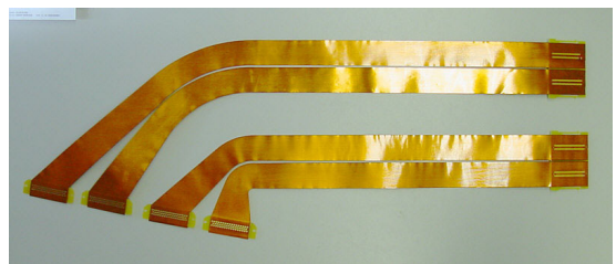
Figure 3.5: Prototype of the seven-layer Kapton-copper cables, that will be used inside the vacuum chamber.
