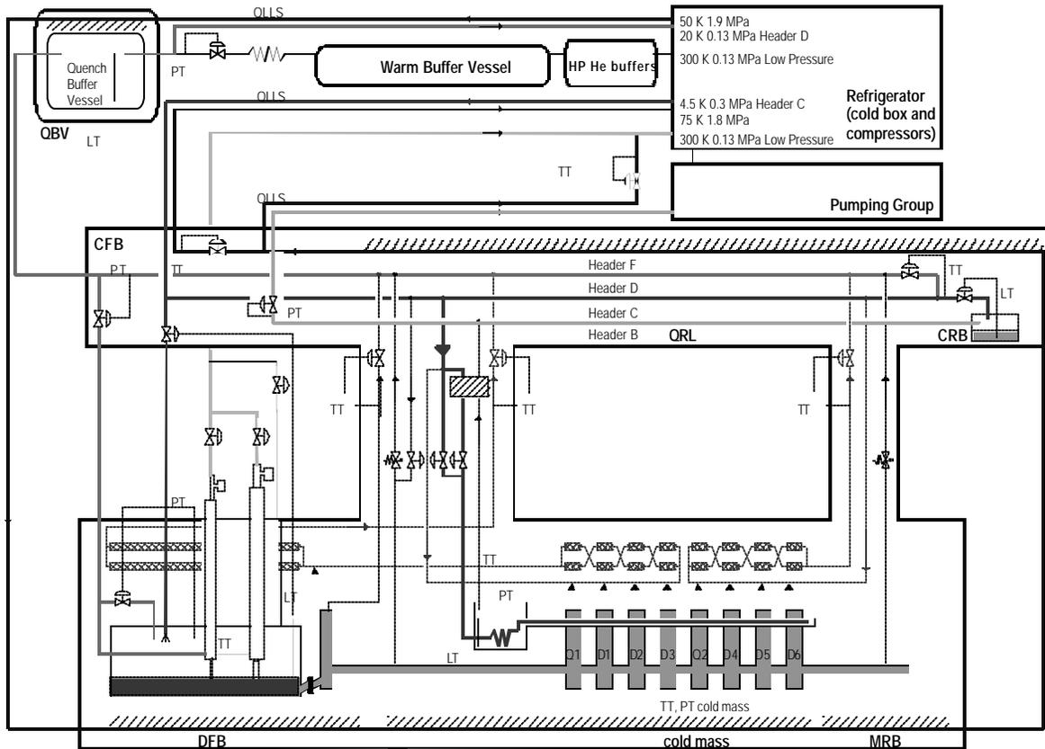
Figure 1 Simplified flow-scheme of the LHC Test String 2
