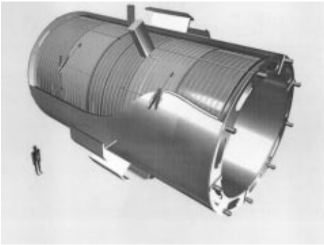
Fig. 4. Perspective view of the CMS coil inside the vacuum tank showing the five modules, the tie-bar suspension system and the thermosiphon cooling circuits outside the mandrels.
