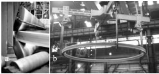
Fig. 2. A 6.8 m diameter ring during two phases of fabrication: (a) seamless ring rolling and (b) transfer of the rolled ring to the quench bath.
