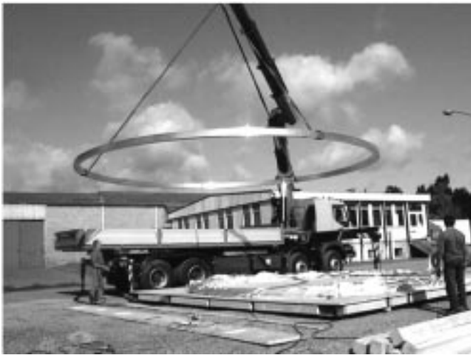
Fig. 3. A pre-machined ring during insertion in the shipment box (courtesy of Dembiermont).
