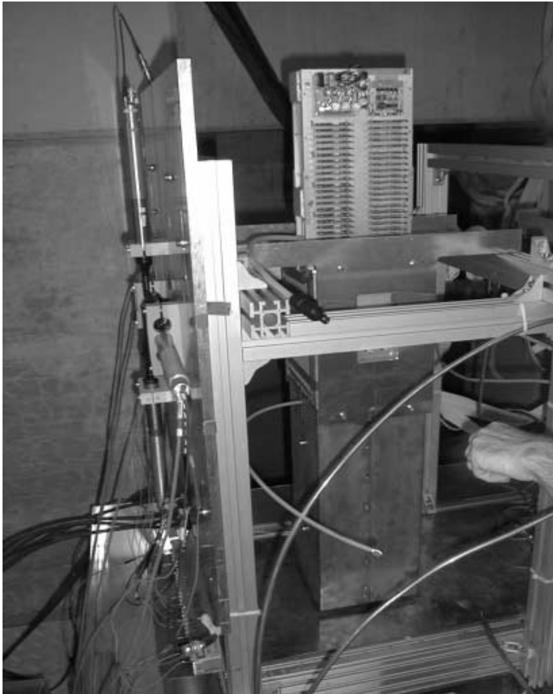
Figure 3: The prototype of KABES 2 double station and tracker in the test beam at CERN SPS in July 2002.
