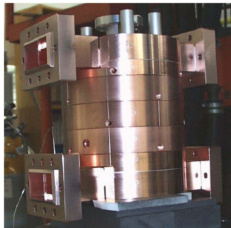
Figure 5: The 6-cell SICA prototype before the high-power tests.
