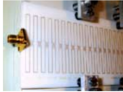
Fig.2: Chopper prototype, double 100 \Omega layout ( Z_0=50 \Omega )
