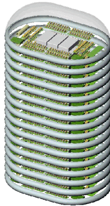
Figure 6. Marx modulator layout. 3' x 5' x 10'
