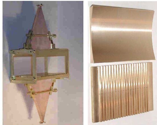
Figure 2: 7-mm resonator (a) prototype and (b) mirrors.
