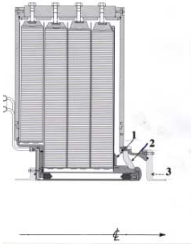
Figure 1: A cutaway view of the DARHT-2 standard cell
