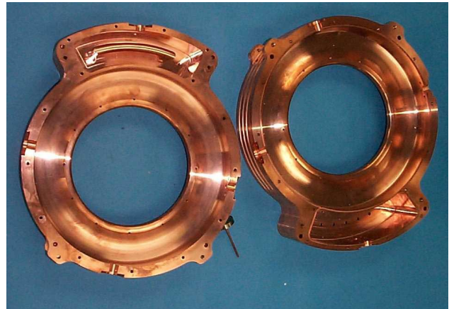
Figure 1: The three-cell copper test model of the \frac{\pi}{2} interleaved RF structure. The open irises will be covered by two beryllium windows of 127 \mu m of thickness and 16 cm of diameter.
