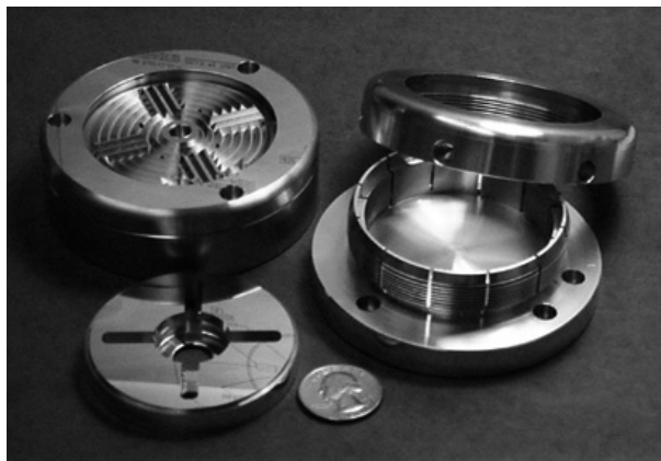
Figure 3: DDS-3 cell with diamond-turning fixtures.
