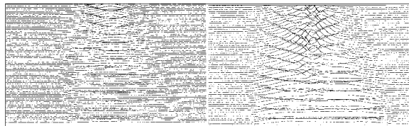
Figure 4 Coherent within-the-bunch vertical motion at AGS injection. Each trace is a new turn. Different parts of the bunch oscillate at different frequencies because of different local coherent tune shift. (because the intensity varies along the bunch) Left is low intensity, 3 \times 10^{12} . Right is high intensity, 10^{13} per bunch.
