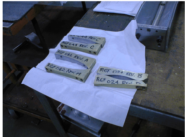
Figure 3: Customized end shims produced on a NC mill to null out error multipoles on Recycler magnets.
