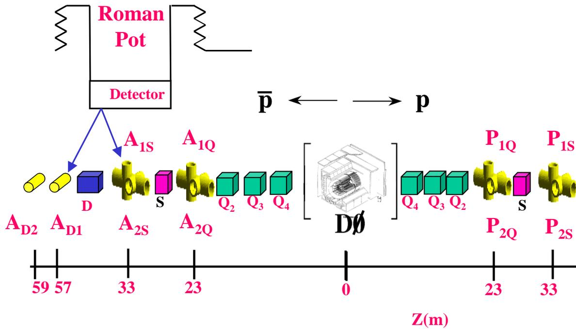
**Figure 1:** Layout of the Roman pot stations and Tevatron components comprising the Forward Proton Detector (see text).
