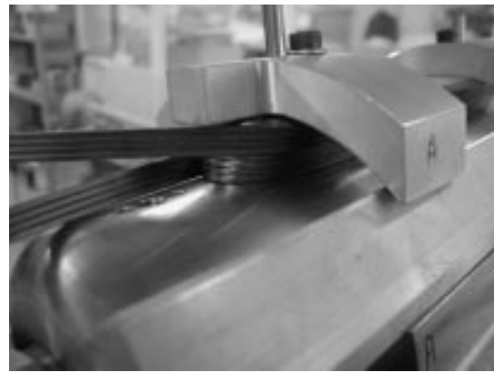
Fig. 3. Counter-winding a coil with a flat cable (MS sextupole model).
