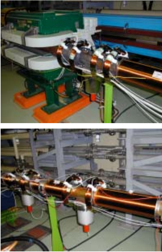
Figure 12 : Solenoids in a NEG pump and bellows section (upper) and in a NEG section (lower). Long solenoids are the bobbin-type solenoids and short solenoids the bobbinless-type solenoids.
