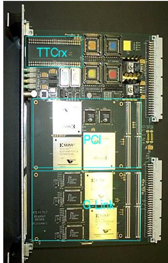
Figure 3: The 6U prototype ROD module.
