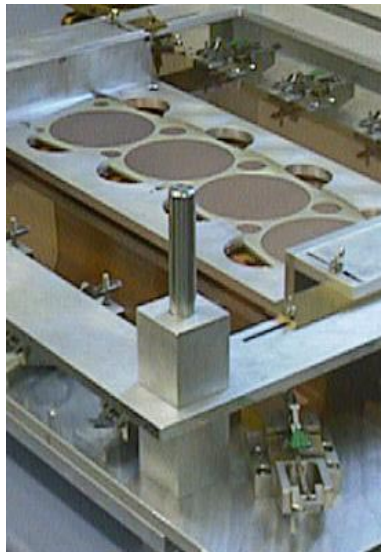
Figure 4: View of the gluing jig. It shows the aligned top frame above the GEM stretched by means of spring-loaded clamps. The aligned spacer frame below the GEM is not visible.
