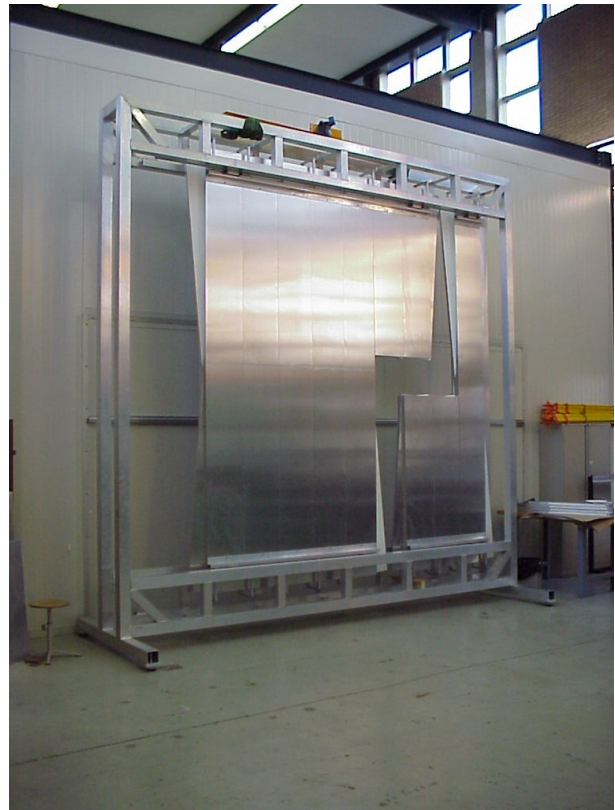
Figure 5.17: Mockup for the study of station assembly.
