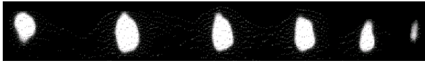
Figure 2: Synchrotron light coming from one of the main dipoles in the microtron. Shown is the light obtained from turn 4 to turn 9 (from right to left)
