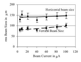
Figure 3: Beam Size vs. Beam Current at high dispersion point in beam delivery line.
