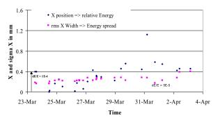
Figure 5: Horizontal position and size of Hall A beam during delivery period. Note the degradation of the spread with time due to uncorrected drifts. Even with drifts, the spread is remarkably small.
