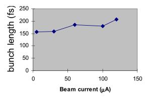
Figure 2: Bunch Length vs. Beam Current out of Injector
