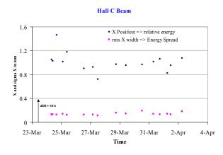
Figure 4: Horizontal position and size of Hall C beam during delivery period. Note that the Hall C beam line provided the energy locking data.
