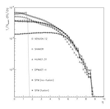
Figure 1: Predictions from different models for the charged pseudorapidity density in central  $(b \leq 3 \text{ fm})$  Pb-Pb collisions at the LHC, taken from [22].
