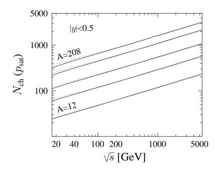
Figure 8: Rapidity density of charged particles at y = 0 for A = 12, 32, 64, 136 and 208 as a function of  $\sqrt{s}$  for central A-A collisions, taken from [44]. The dotted line is the result of (27), the solid line is the result of a more rigorous calculation.
