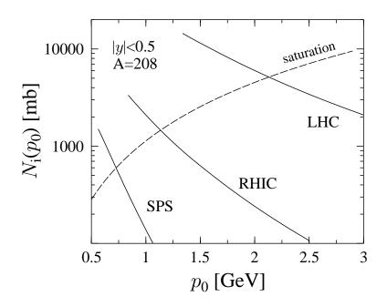
Figure 7:  $N_{AA}(b = 0, p_0, \sqrt{s})$  with  $p_T \ge p_0$  and |y| < 0.5 for A = 208 as a function of  $p_0$  at  $\sqrt{s} = 5500$  (LHC), 200 (RHIC) and 17 (SPS) GeV per nucleon, taken from [44]. The dashed curve is  $p_0^2 R_A^2$ .
