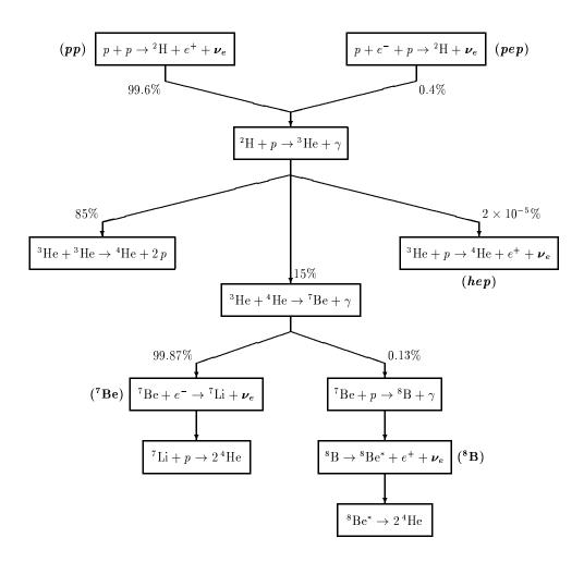
Fig. 1: The pp cycle (the figure is taken from Ref. [17]).
