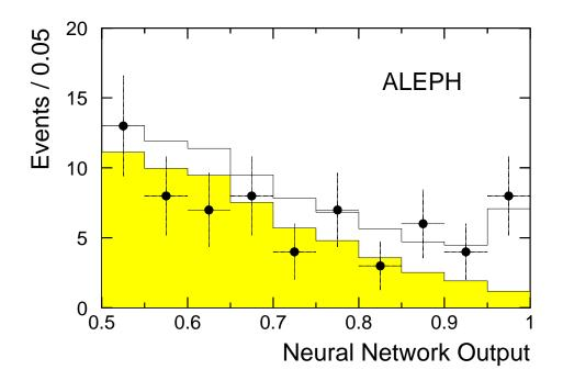
Figure 5: Neural network output from the  $q\overline{q}q\overline{q}$  selection for data and Monte Carlo simulation. The grey histogram shows the expected background, and the hollow histogram shows the expected  $\mathcal{NC2}$  signal.
