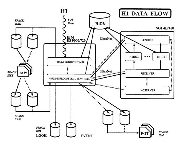
A fast data link is required connecting the mainframe and the workstations that became available by an UltraNet installation at DESY in summer 1991. A (memory-to-memory) transfer rate of 7.5 MB/s has been measured using two-way stripe mode and two IBM BMPX channels, at a reasonably small CPU load on both hosts due to protocol evaluation.
