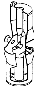
Fig. 2. A two-gap superconducting niobium resonator which was constructed and tested at ANL by Delayen, et al. [14].
