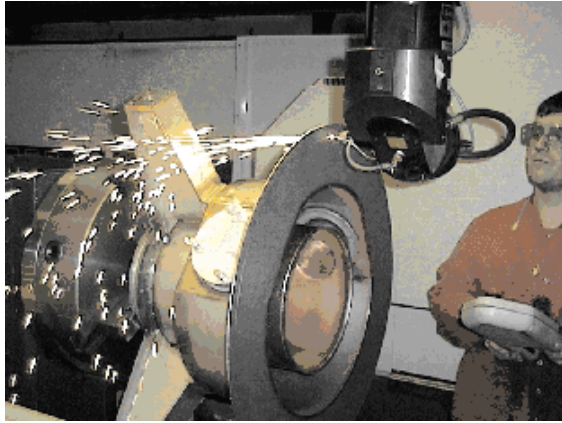
Figure 4: Laser cutting the He tank at the good dimension. The cutoff is visible inside the tank.
