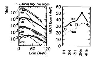
Figure 3: Light charged particle characteristics for data (markers:  $-0.5 \le \cos\Theta_{\rm cm} \le 0.5$ ), SMM (dashed-lines:  $-0.5 \le \cos\Theta_{\rm cm} \le 0.5$ ) and EES (solid-lines): left): c.m kinetic-energy spectra, right): c.m mean kinetic-energy.
