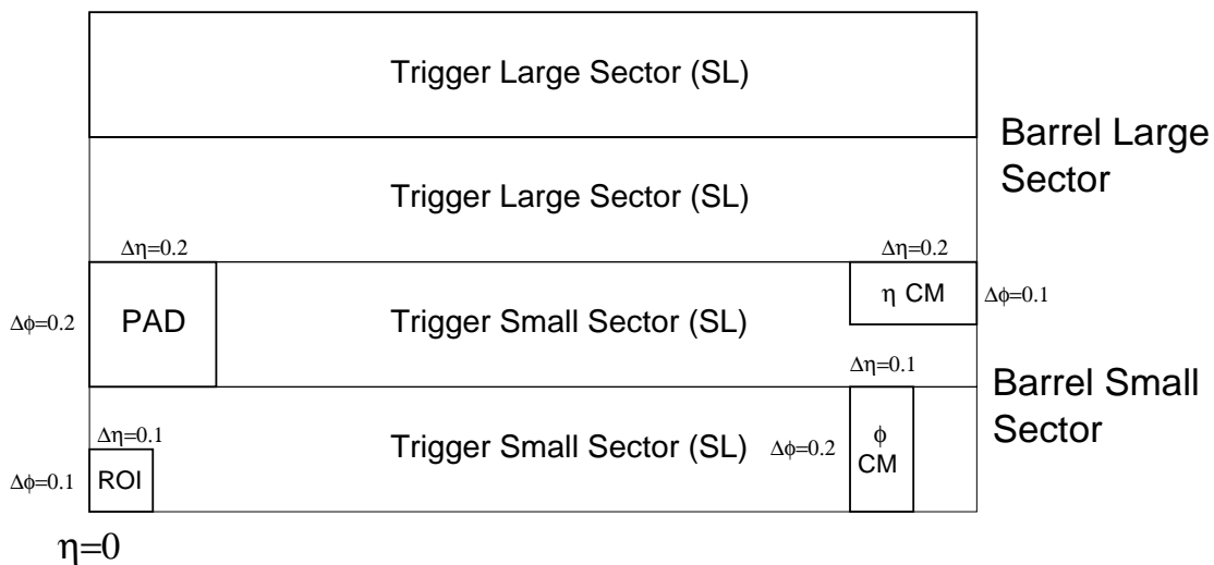
Figure 11-4 Barrel trigger segmentation. Also indicated in the figure are the areas covered by \eta and \phi CM boards, by an ROI, by a Pad Logic (PL) board and by a Sector Logic (SL) board.
