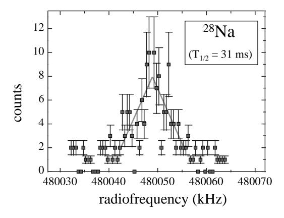
**FIGURE 2.** A recorded (reconstructed) peak for  $^{28}$ Na ( $T_{1/2} = 30.5$  ms). This measurement corresponds to 64 (random) frequency steps of 320 ms each. The center frequency of about 480,050 kHz is derived from a triangular fit [15] and corresponds to harmonic number 2342 of the cyclotron frequency of  $^{28}$ Na in the 0.37359 T field at a beam energy of 60 keV. The mass resolution is 47,860.
