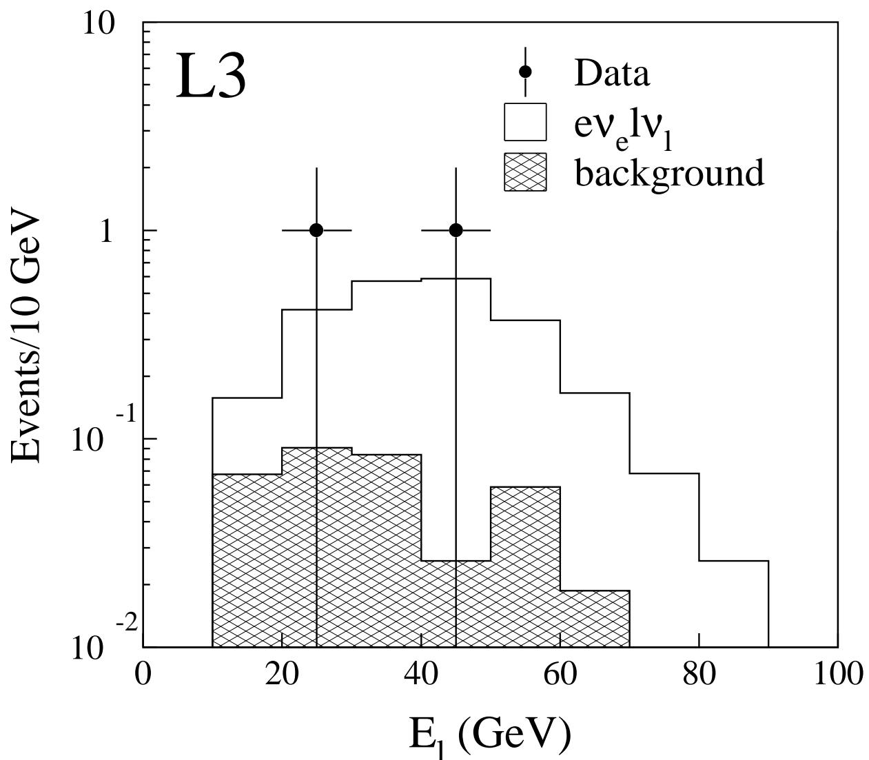
Figure 5: The energy spectrum of the selected leptonic candidates. The hatched histogram represents the background, the open histogram shows the fitted signal (2) from  $e\nu_e \ell \nu_\ell$  final states.
