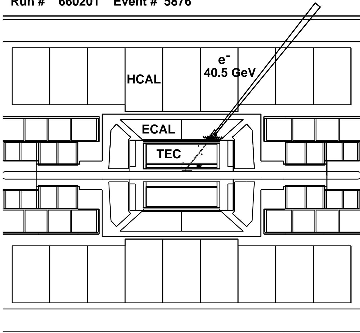
Figure 4: A  $e^+e^- \rightarrow e^+\nu_e W^-$ ,  $W^- \rightarrow e^-\bar{\nu}_e$  candidate event. In the upper hemisphere the 40.5 GeV electron is detected in the tracking chamber and in the electromagnetic calorimeter where the pulse heights represent the electron energy deposition . No significant energy deposition is observed in other subdetectors since the positron escapes in the beam pipe.
