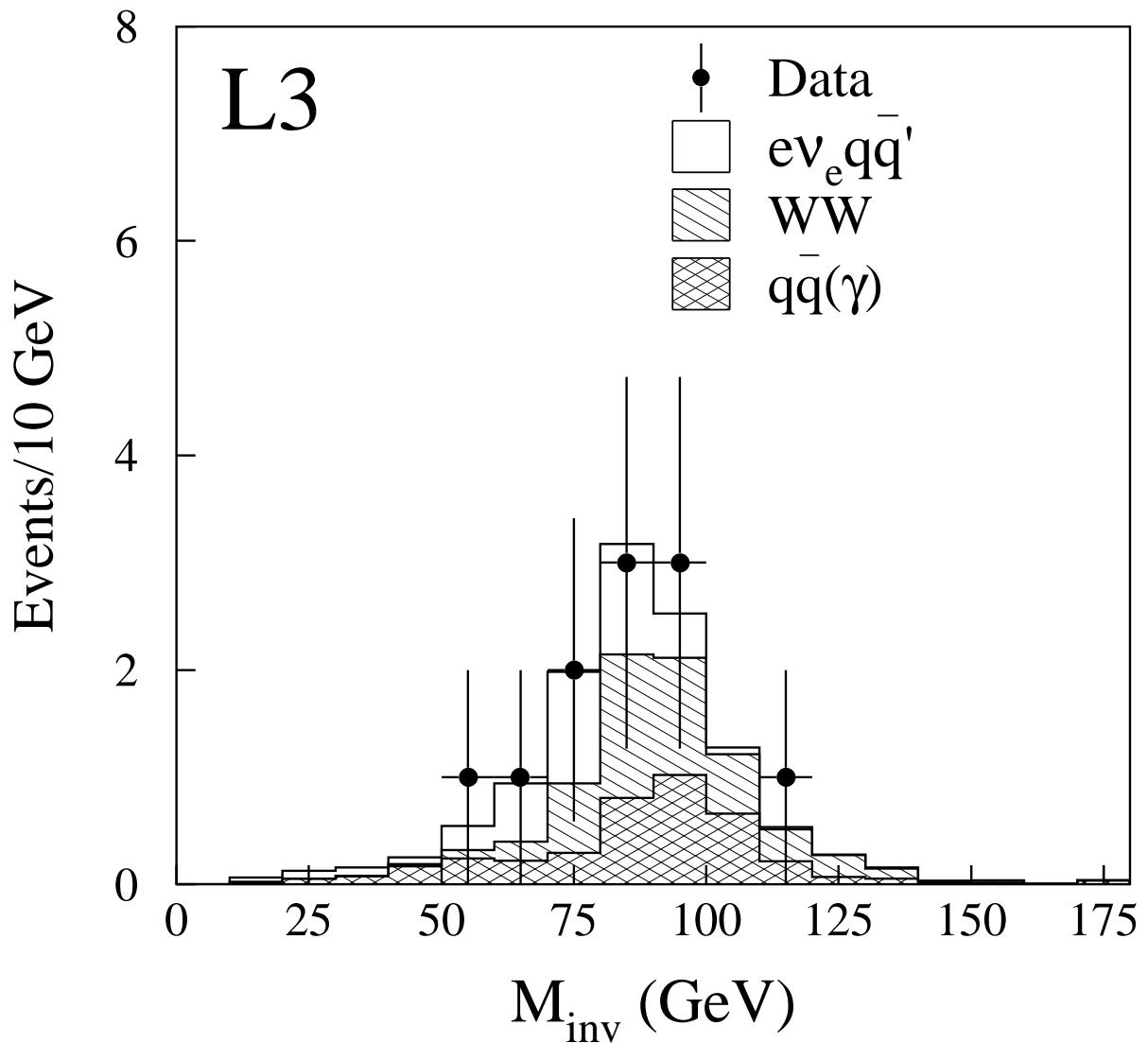
Figure 7: The jet-jet invariant mass spectrum,  $M_{inv}$  of the selected hadronic candidates for the combined data sample. The hatched histogram represents the background, the open histogram shows the fitted signal from  $e^+\nu_e q\bar{q}'$  final states.
