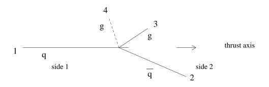
Figure 4: Dipoles in ARIADNE. The dashed line represents the radiation of a second gluon.
