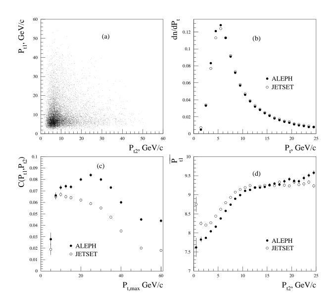
Figure 1: 1992 ALEPH data and reconstructed JETSET events. a) Scatter plot of  $P_{t1}$  versus  $P_{t2}$  for ALEPH data. b)  $P_t$  distribution for events with  $P_{t1}, P_{t2} < 25 \text{ GeV/c. c}$ ) Correlation as a function of  $P_{t,max}$  when only events with  $P_{t1}, P_{t2} < P_{t,max}$  are accepted. d) Average  $P_{t1}$  as a function of  $P_{t2}$  for the events in (b).
