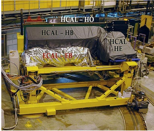
Figure 2. An overview of the H2 test beam area showcasing the HB, HE, HO, and ECAL EB components, all meticulously mounted on a versatile moving platform [10].
