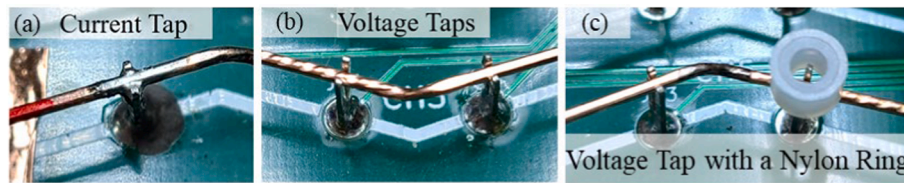
Fig. 13. Close up images of the (a) soldered current contact and (b) a typical pair of voltage taps at a cable edge. The dented face along the left-hand side of straight section is the inside face of the cable. (c) is an optional modification using a nylon ring to help secure the wire in the Y-slot.
