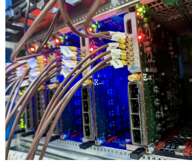
(b) Picture of one of the \mu TCA crates with GLIB cards and input signals [66].
