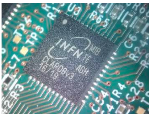
Figure 5.15: (Left) CLARO ASIC with its packaging. (Right) Block schematic of a CLARO channel. The purpose of the dummy amplifier is to give each channel a differential structure, improving the power supply rejection ratio and allowing DC-coupled input to the discriminator [166].
