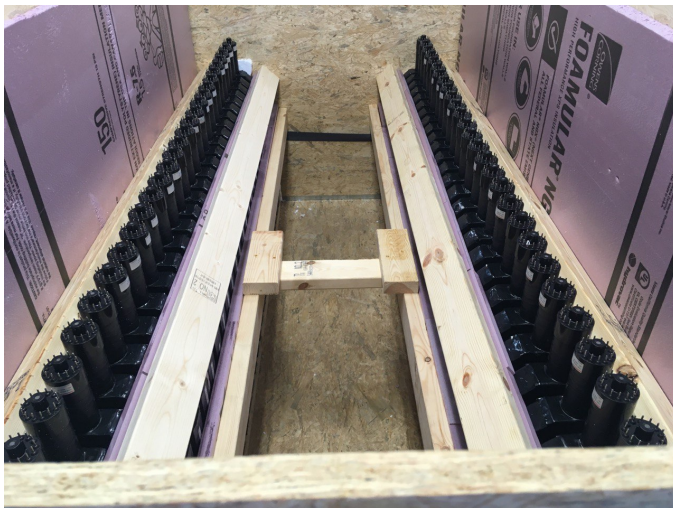
Fig. 19: OD scintillation units at the University of Alabama, ready to be shipped to CERN.
