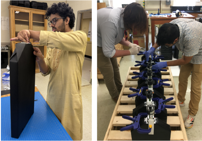
Fig. 18: Work on OD scintillation units at the University of Alabama. As of end of August, all 60 slabs has been wrapped, and the calibration LEDs have been glued in. Roughly half of the slabs have the PMTs glued in. From left to right: Alabama students U. Ullah, B. Davis, A. Upreti.
