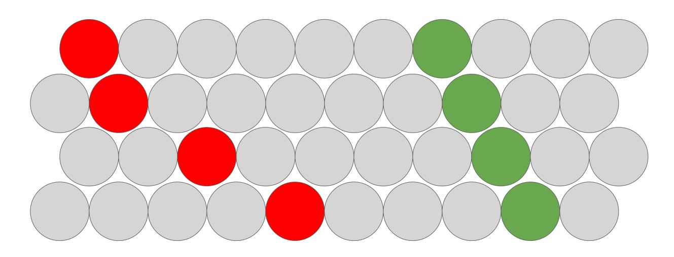
• Road: pre-defined set of MDT tubes compatible with a high- $p_{\tau}$  muon track
