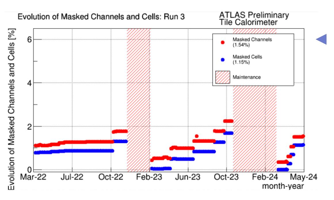
Continuous data quality activities and maintenance campaigns keep the fraction of non-functional readout channels below 2%.
