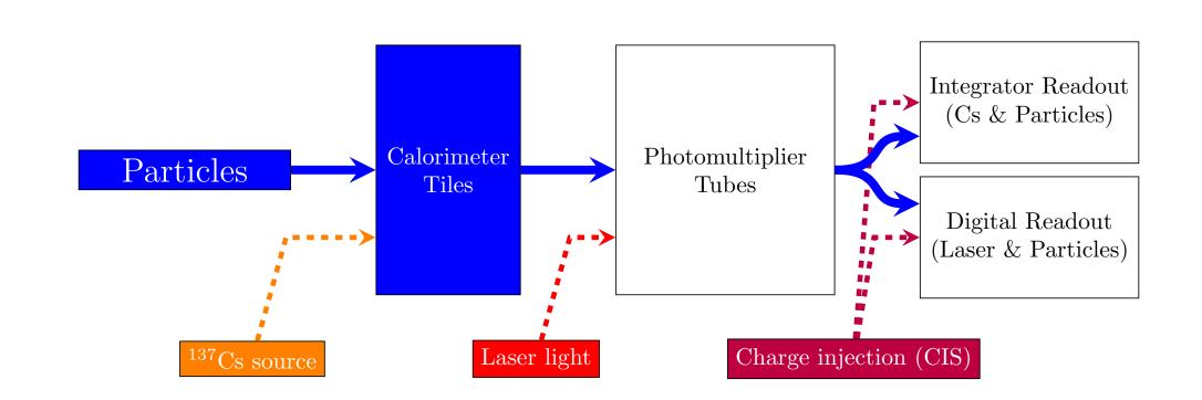
Charge-injection calibrates the readout electronics.
