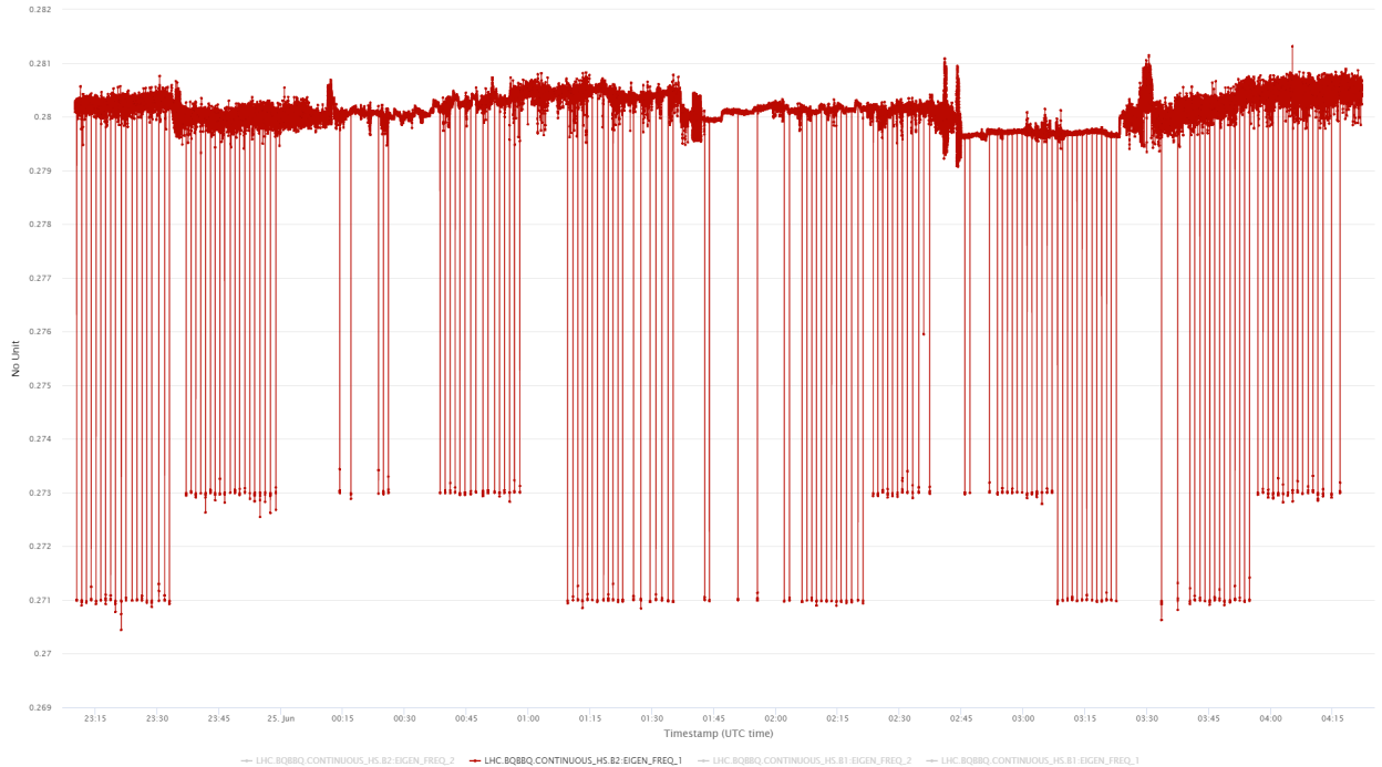
Figure 1: Horizontal tune as measured from the BBQ system in Beam 2 during the duration of MD6863.
