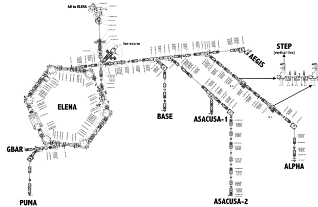
Figure 1: ELENA ring with the extraction lines.
