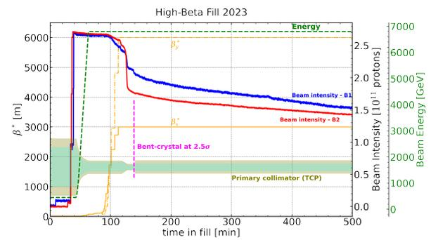
Figure 5: Beam intensity evolution during a high- $\beta^*$  fill.
