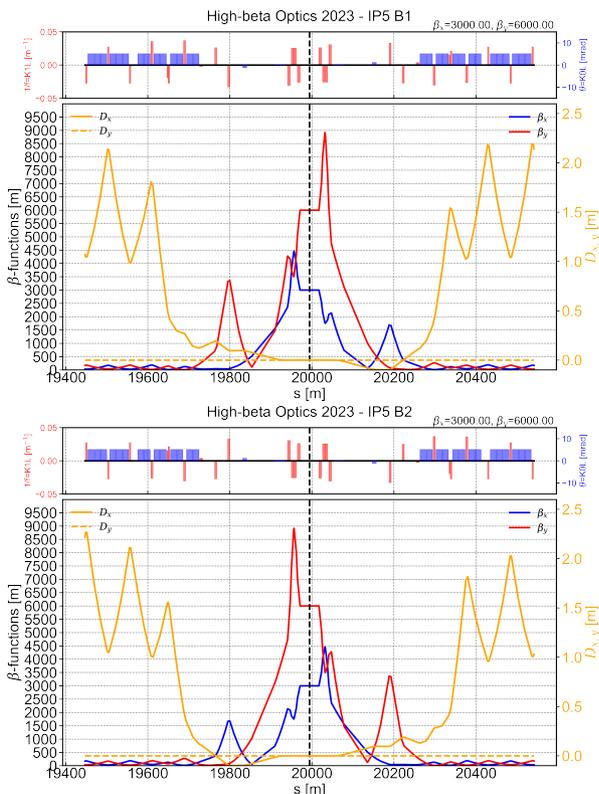
Figure 2: The 3/6 km high-beta optics at IP5 for B1 (top) and B2 (bottom).
