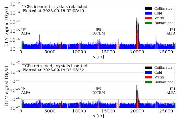
Figure 6: Loss pattern along the LHC ring during the high- $\beta^*$  3/6 km fill, using a standard TCP (top) or a bent-crystal (bottom) as primary collimator.
