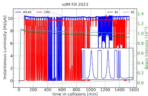
Figure 4: Beam intensity and instantaneous luminosity evolution in ATLAS and CMS experiments during a long vdM fill in June 2023. Inset: zoom in a period with two successive Vernier scans of the beams in  $x$  and  $y$  planes up to  $6\sigma$ .
