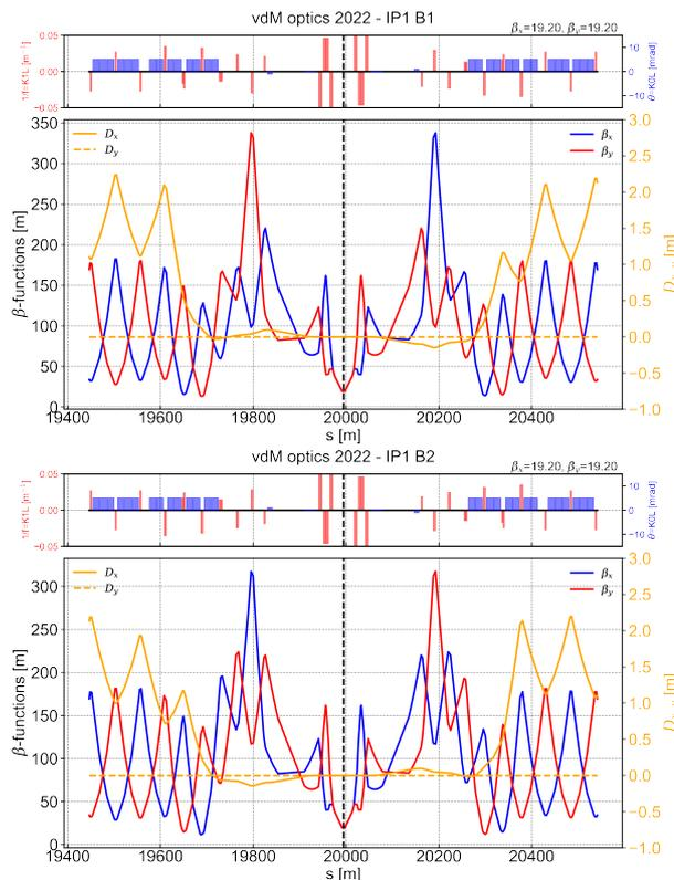
Figure 1: The vdM optics for the insertion around IP1 for B1 (top) and B2 (bottom) at a  $\beta^*$  of 19.2 m.
