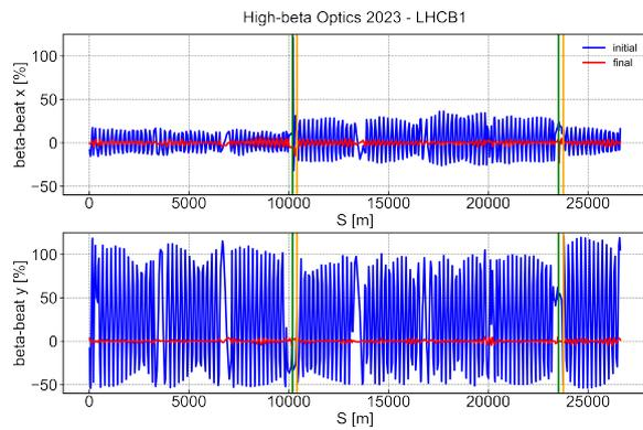
Figure 3: Beta-beating of B1 before and after all corrections for the  $x$  (top) and  $y$  (bottom) planes for the 3/6 km optics. The green lines indicate the location of the IPs and the orange the RP detectors. Similar performance was observed for B2.
