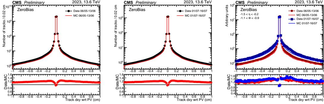
**Figure 5:** Distance of closest approach with respect to the primary vertex of tracks passing the selection described in the text: for the first (left) and the second (middle) period of 2023 in the full geometric range, with a comparison of the two periods in the pixel tracker region affected by the readout failure (right). Results are taken from [9].
