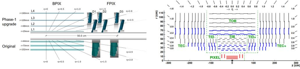
**Figure 1:** Layout of the CMS tracker. The figure on the left, the layout of the pixel subdetector, is from [5], the figure on the right, the overall layout of the tracker, is from [3].
