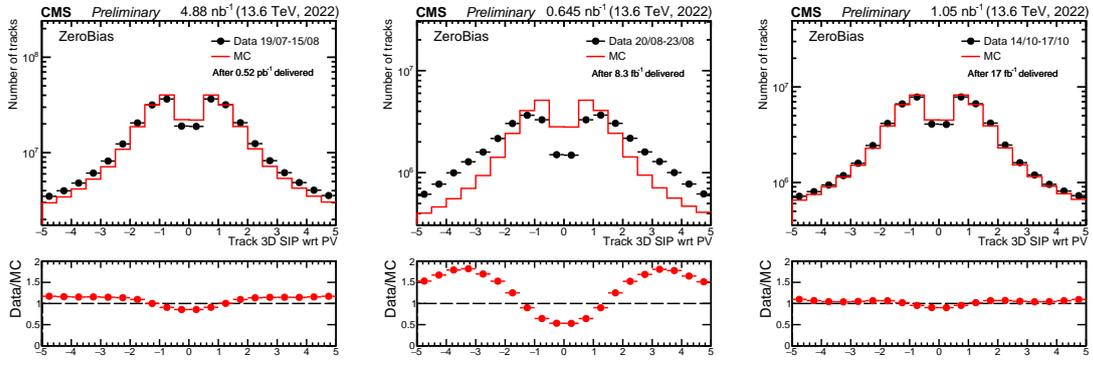
**Figure 2:** Significance of the 3D impact parameter in data and Monte Carlo for the different data-taking periods and after the integrated luminosity delivered since the replacement of the first layer of the Barrel Pixel Detector indicated in the figures. Results are taken from [8].
