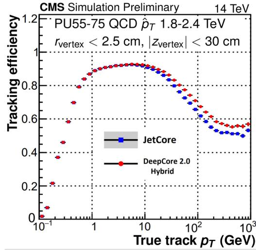
**Figure 7:** Reconstruction efficiency of the tracks inside the core of jets with high transverse momentum  $p_T$  (selected as described in [12]) as a function of the  $p_T$  of the tracks when the default (in blue) or DeepCore 2.0 hybrid (in red) iteration for tracking inside of high- $p_T$  jets is used. Results are taken from [12].
