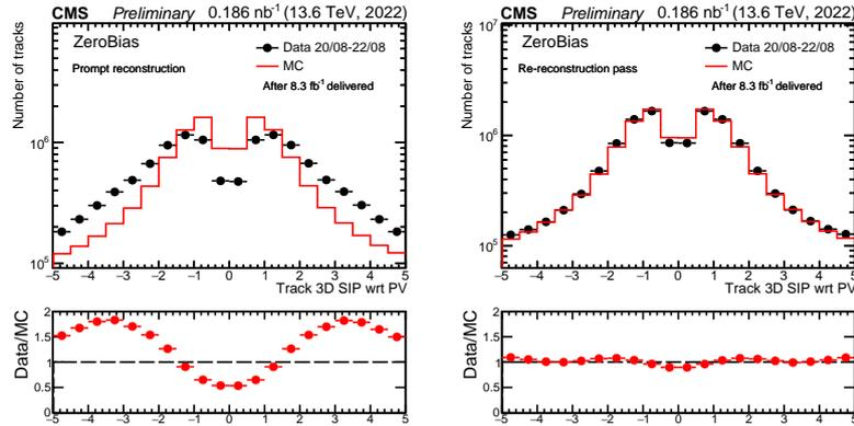
**Figure 3:** Significance of the 3D impact parameter distribution in data and Monte Carlo selecting only the tracks in the period in the figure for which the updated reconstruction was performed. Results are taken from [8].
