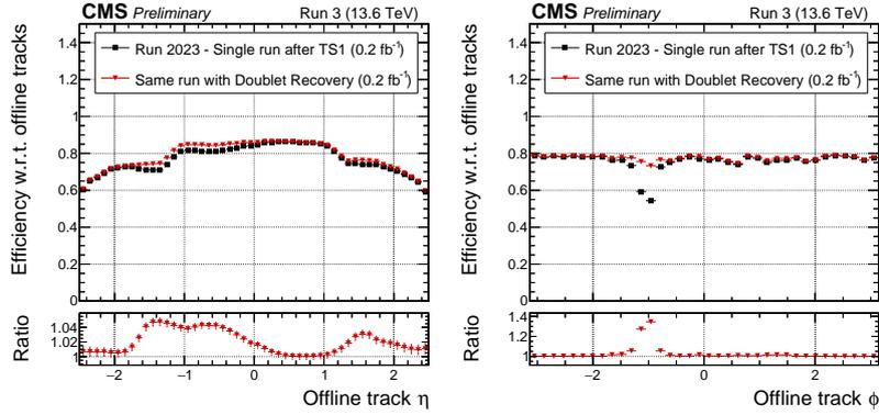
**Figure 6:** Reconstruction efficiency at High Level Trigger with respect to the offline reconstruction as a function of  $\eta$ , on the left, and  $\phi$ , on the right, with and without the pixel doublet recovery iteration. Results are taken from [11].
