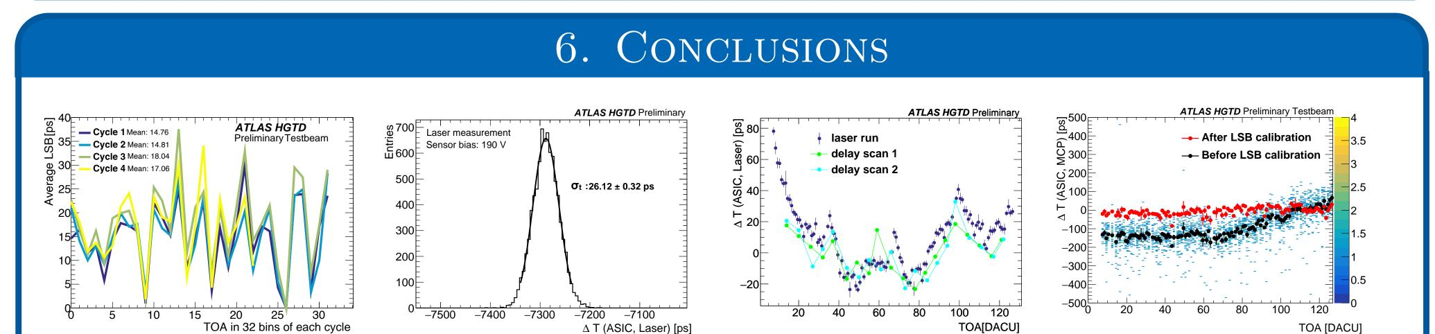
After the LSB was estimated with the MCP reference and the time-walk correction being applied, the time difference distribution was generated and a gaussian fitting was performed. As shown in the figure, the time resolution of 45.8 ps for the pixel of interest in the middle of the array (row 7, column 7) is obtained. The linearity of the TOA LSB is verified by the inset plot.
