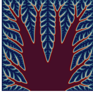
Figure 9: Optimized density \tilde{\rho} for thermal compliance problem with deterministic heat source and volume constraint 50% (i.e., \gamma = 0.5 ). The length parameter in the PDE filter is set to r = 0.02 .
