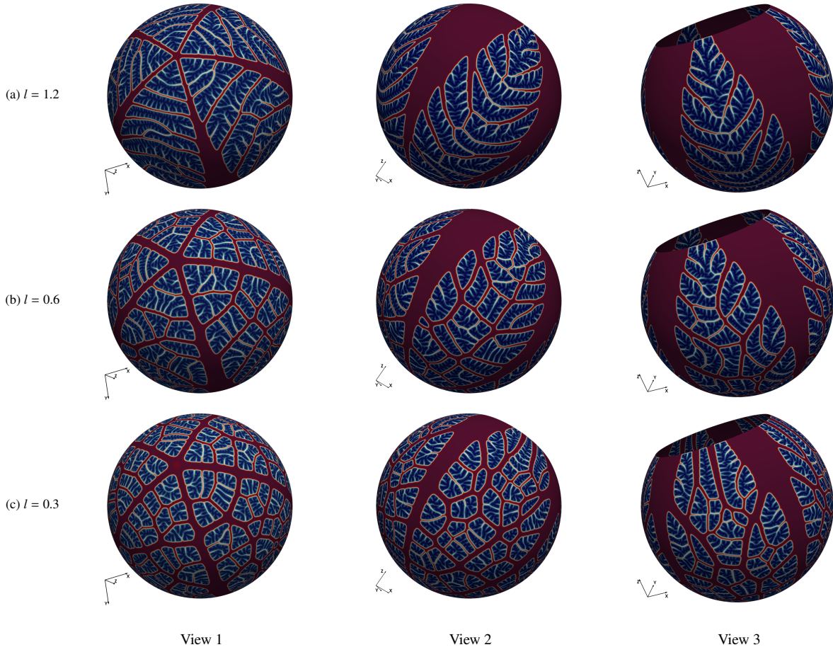
Figure 13: Optimized density distributions \bar{\rho} for thermal compliance problems with stochastic heat source, different correlation lengths, and volume constraint 50% on a cut sphere. The length parameter in the PDE filter is set to r = 0.02 . The stochastic fields are isotropic. The values of the objective function are j_{(a)} = 39.74 , j_{(b)} = 17.75 , and j_{(c)} = 7.61 .
