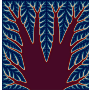
Fig. 9. Optimized density \bar{\rho} for thermal compliance problem with deterministic heat source and volume constraint 50% (i.e., \gamma = 0.5 ). The length parameter in the PDE filter is set to r = 0.02 .
