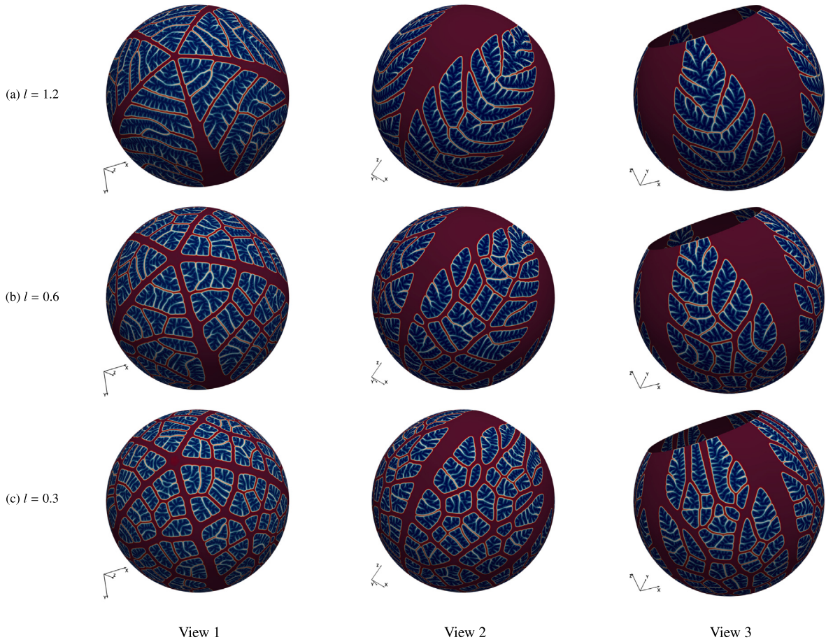
Fig. 13. Optimized density distributions \bar{\rho} for thermal compliance problems with stochastic heat source, different correlation lengths, and volume constraint 50% on a cut sphere. The length parameter in the PDE filter is set to r = 0.02 . The stochastic fields are isotropic. The values of the objective function are j_{(a)} = 39.74 , j_{(b)} = 17.75 , and j_{(c)} = 7.61 .
