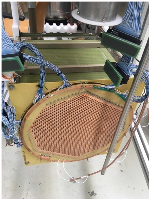
Figure 7. Photo of the LARISA 3-plane anodic readout system mounted on the TPC. The Collection plane is visible in the foreground, as the cables carrying the signal from strips and the bias on each plane. The field cage can be seen in the background.
